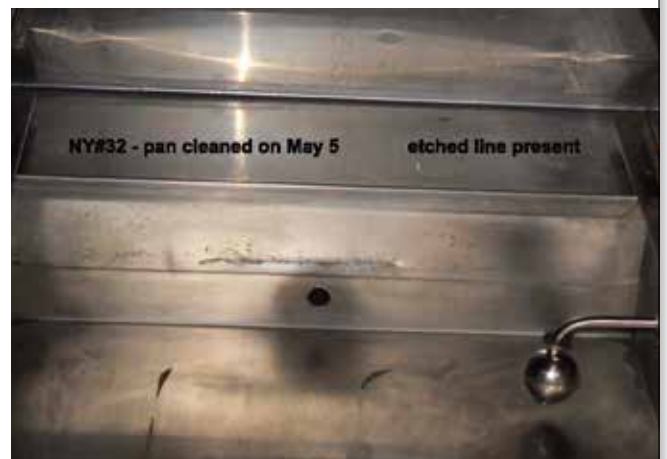
After Vulcan installation — pan area is now completely scale-free. There is a slight indentation into the pan at the waterline.
