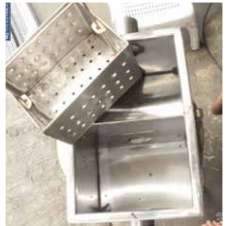
Grease traps have reduced odors and more consistent, less cluttering grease.
