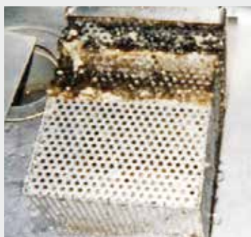
The status after being used without cleaning since the installation in June (no adhered materials are seen on the portions usually contacting with water).
